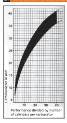
The most important aspect of a carburetor is it's size. The value of the carburetor size is based on the diameter of the induction port (for example, PHBG 19 = 19mm induction port diameter). Depending on how much the motor had been modified, a larger induction diameter guarantees a real power increase in higher rpm's, while a smaller carburetor diameter results in better acceleration.
